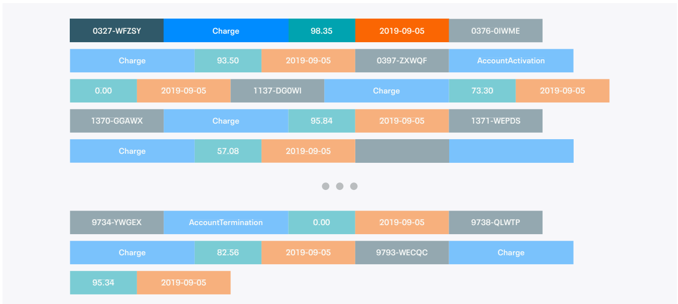
Figure 14. A portion of the billing events table, represented in a row-oriented storage format, with field values from the same record adjacent to one another
